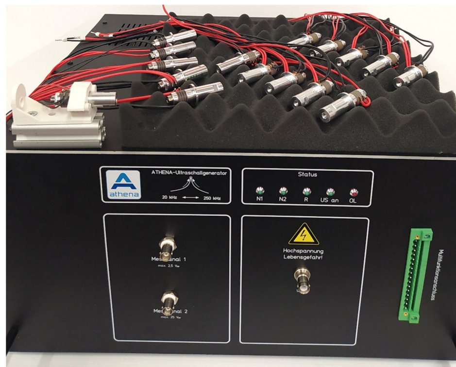
Figure 3. Series of assembled transducers with PZT and lead-free piezoelectric ceramics, plastic mounting bracket, and ATHENA ultrasound generator being used for resonance-controlled operation and measurements.
